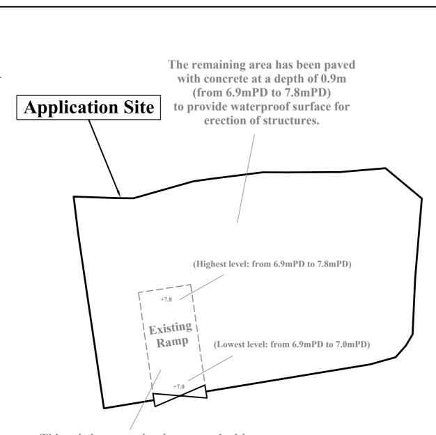
This existing ramp has been paved with concrete at a depth of 0.1m to 0.9m to provide waterproof surface for maneuvering.
